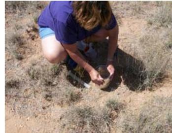
Figure 7: Beth placing cylinder in Black grama grassland plot to time speeds of water into the soil.
